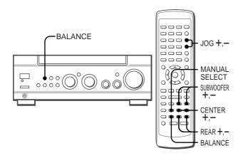
The unit is equipped with a built-in test signal generator called a noise sequencer for easy balance adjustment of all five channels. The sequencer outputs a noise signal that "travels" from channel to channel, enabling the simple adjustment of sound level to achieve the same apparent loudness, at your listening position, from each channel.
